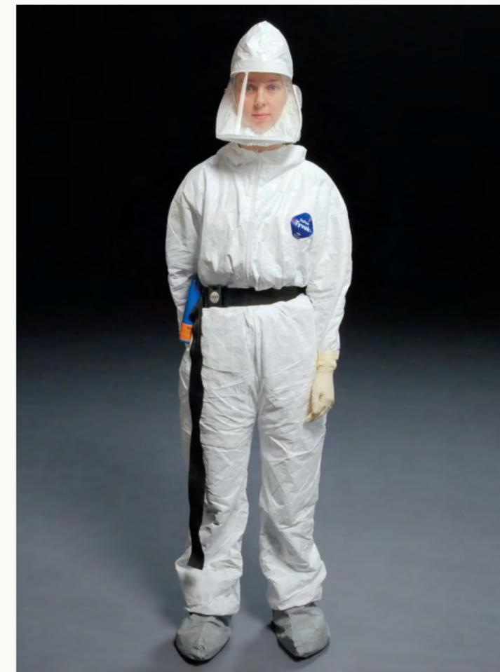
This photograph depicted a Centers for Disease Control and Prevention (CDC) scientist demonstrating how one is to properly wear personal protective equipment (PPE) in appropriate laboratory settings. This PPE outfit included the suit, double gloves, and a powered air purifying respirator. Photo: CDC / Unsplash
