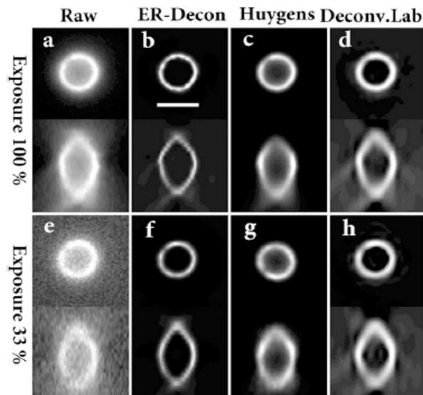
Fig. 1: Synthetic example for illustration of the performance of the entropy-based regularization (ER) deconvolution of Arigovindan *et al.*<sup>2</sup> (image from corresponding publication).
